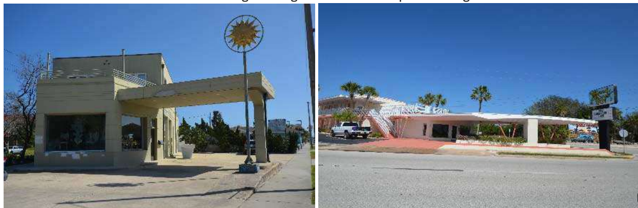
Projecting Sign (Bracket Sign) – a sign which is affixed and displayed perpendicular to any building wall or structure.
