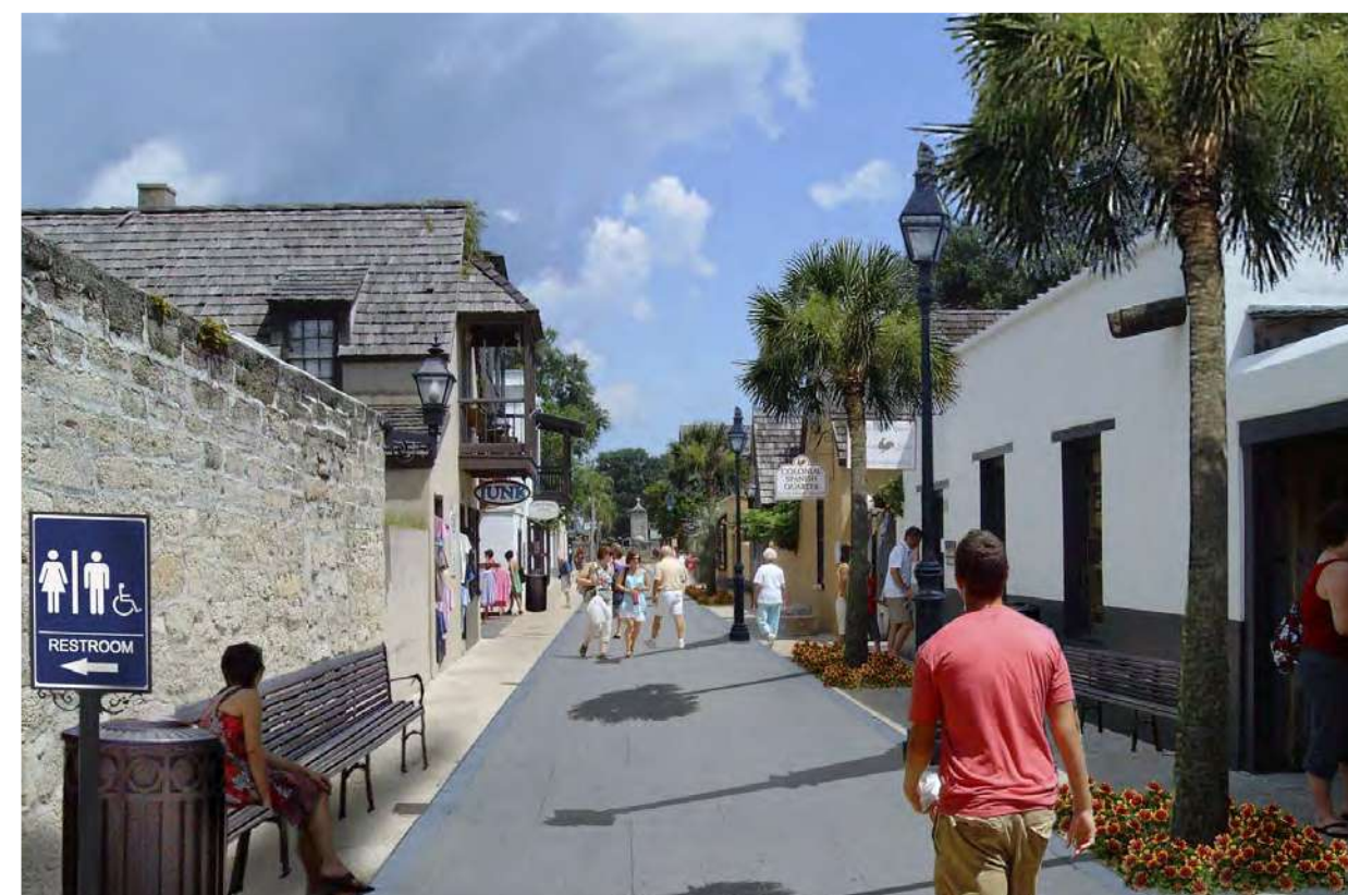
AFTER Colored coquina concrete, cut into large rectangles, along with a flush granite curb creates visual interest for the expansive hardscape. Cabbage palms and historic lighting complete the renewed streetscape.
